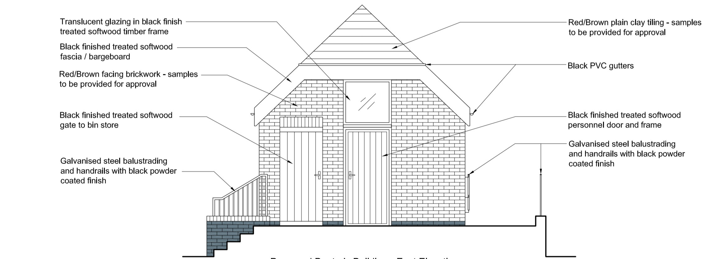
Proposed Boater's Building - East Elevation Scale 1/50
